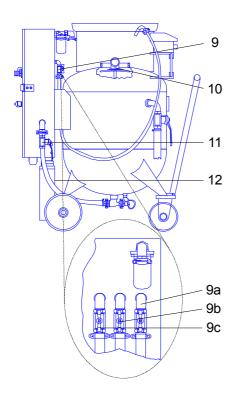
**Switching ZW (11) – Equipment (511)**: It allows to switch over from blasting to cleaning or to drying at the machine.
